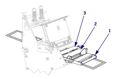
**8.** Push the media forward until it passes under the printhead assembly (1), under the snap plate (2), and then over the platen roller (3).
